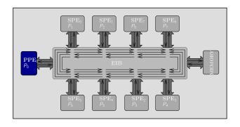
One Power core (PPE) P<sub>0</sub> standard processor, direct access to memory and L1/L2 cache
