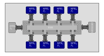
▶ Eight Synergistic Processing Elements (**SPE**s)  $P_1, \ldots, P_8$  256-kB Local Stores, dedicated asynchronous DMA engine
