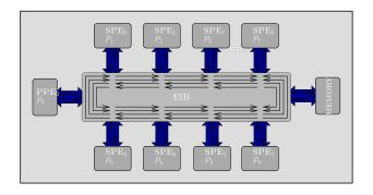
$\blacktriangleright$  Bidirectional communication link between an element and the EIB bandwidth  $\mathrm{bw}=25 GB/s$
